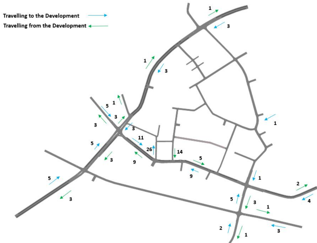
Figure 7.7: PM Peak Development Traffic Distribution
